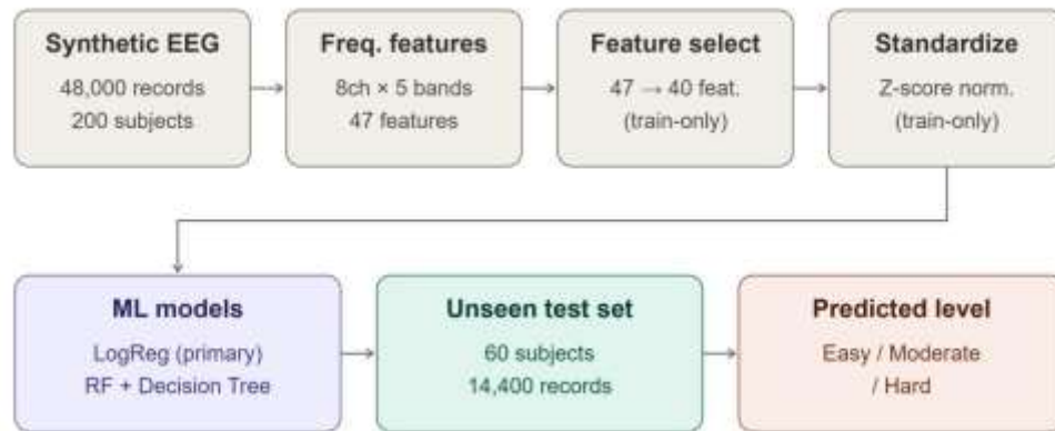
Fig. 1. Proposed subject-independent frequency-domain EEG classification pipeline.
