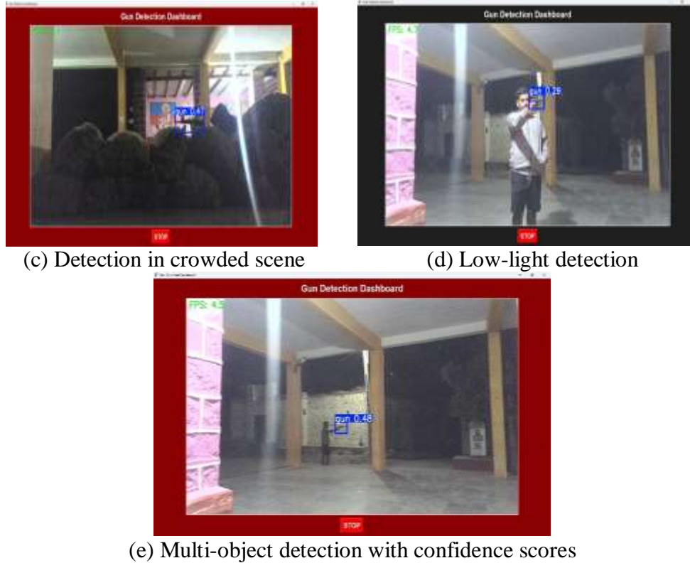
Fig. 5: Real-time firearm detection results from YOLOv12m. Bounding boxes, class labels, and confidence scores are over-laid on surveillance video frames.
