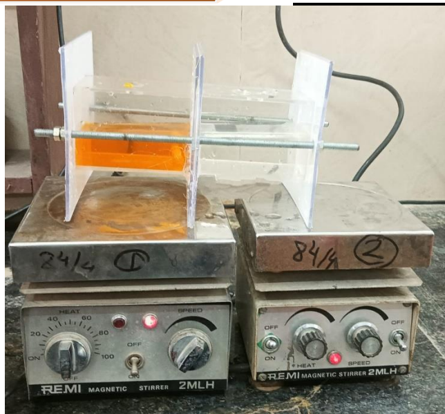
Fig.3 Polymer Inclusion Membrane set up
