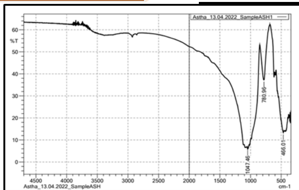
Fig. 6 (B) FTIR Spectra of Sugarcae Bagasse Ash
