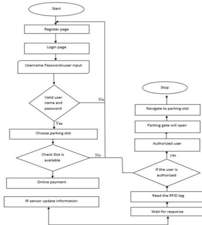
Figure 3: Flow chart for Overall System
